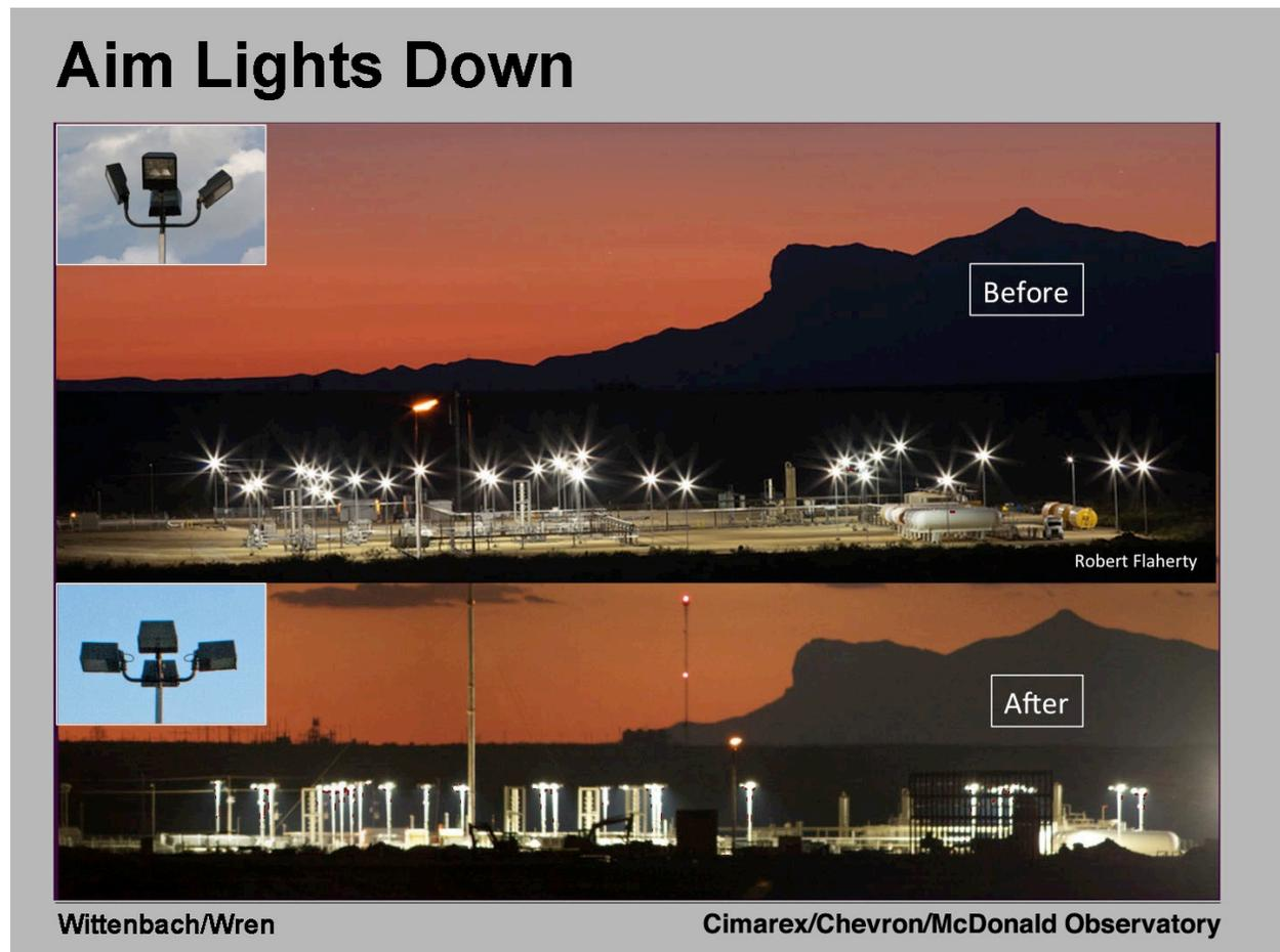
Construction and permanent lighting should be mounted and directed to focus light only on the intended area, and to avoid light spill and offsite light trespass. Lights pointing upward or horizontally should be avoided.
